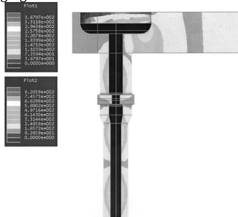
Fig. 2. Coupler electric fields in V/m for 1 W average input power
